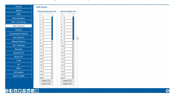
If roaming operator list is left empty, FMB964 will automatically detect home operator. If home operator is written to the roaming operator list, it will still be detected as home operator. Any operator not in the roaming operator list (except the home operator) will be recognized as unknown operator and FMB964 will work in Unknown mode (make sure it is configured to allow data sending – GPRS context is enabled).
