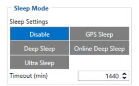
When in GPS sleep mode, FMB964 turns the GPS module off and continues making new periodic records. As a result power usage decreases, in turn saving vehicle battery.
