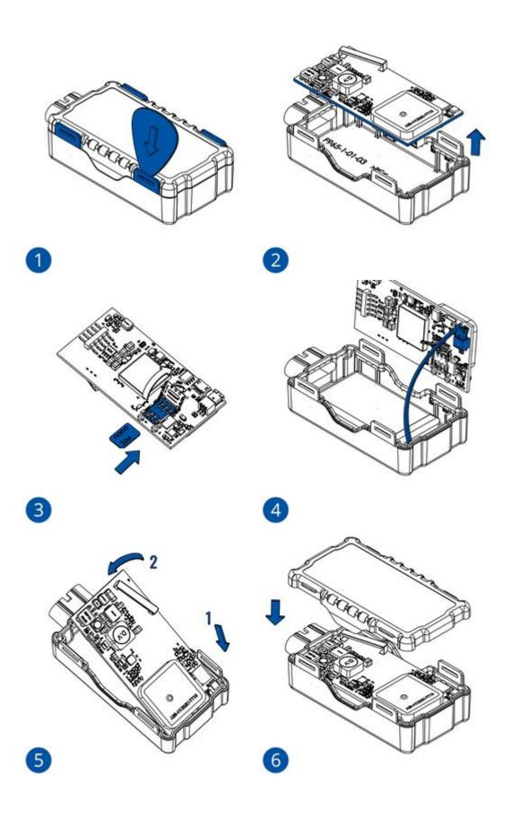
Nano-SIM card insertion/removal must be performed when device is powered off
