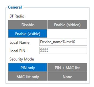
General functionality configures Bluetooth to work in slave mode. This mode allows any external device to connect to FMC003.
