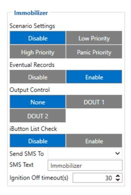
If *DOUT Control* is disabled, the scenario will only generate events without digital output activation. If *DOUT Control* is enabled DOUT1/DOUT2 turns ON if ignition turns ON (*Ignition Source* is
