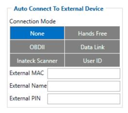
Auto connection functionality configures FMC234 as master device, which allows connecting FMC234 to an external device. FMC234 currently supports these modes:
