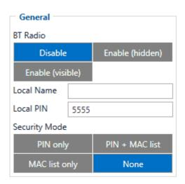
General functionality configures Bluetooth @ to work in slave mode. This mode allows any external device to connect to FMC234.
