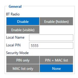
General functionality configures Bluetooth to work in slave mode. This mode allows any external device to connect to FMC640.
