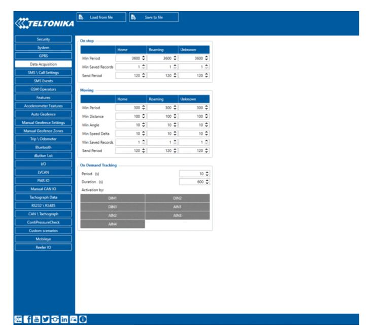
There are three available options for the activation source of tracking on demand - DIN/AIN or both (devices that support multiple DINs/AINs allow choosing which DINs/AINs to use). Note that, these inputs will work as buttons, rather than switches, and are used to trigger the functionality, the duration of tracking on demand will not be extended if the activation source status is high for a period of time.
