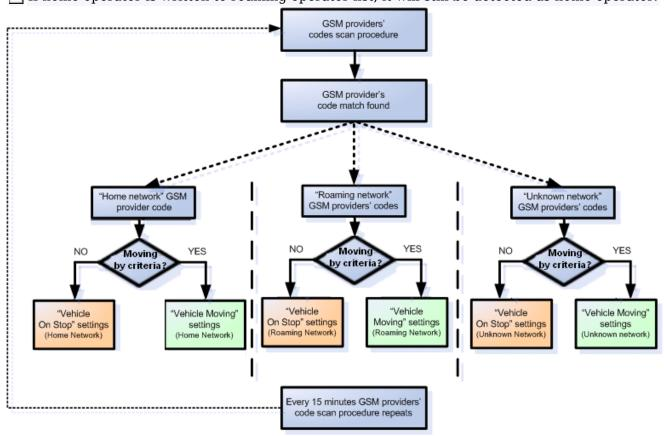
Operator search is performed every 15 minutes. Depending on current GSM operator Home, Roaming or Unknown mode can be changed faster than every 15 minutes. This process is separate from operator search. Movement criteria are checked every second.
