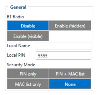
General functionality configures Bluetooth® to work in slave mode. This mode allows any external device to connect to FMC800.
