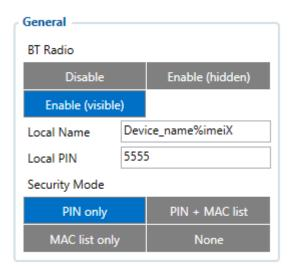
General functionality configures Bluetooth @ to work in slave mode. This mode allows any external device to connect to FMC800.
