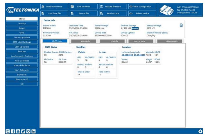
Various <u>Status window</u> tabs display information about <u>GNSS</u>, <u>GSM</u>, <u>I/O</u>, <u>Maintenance</u> and etc. FMC800 has one user editable profile, which can be loaded and saved to the device. After any modification of configuration the changes need to be saved to device using **Save to device** button. Main buttons offer following functionality:
