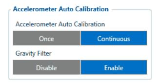
Users can disable or enable Accelerometer Auto Calibration and Gravity Filter features. Under Accelerometer Auto Calibration settings, user can choose:
