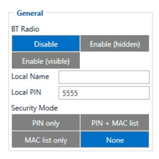
General functionality configures Bluetooth to work in slave mode. This mode allows any external device to connect to FMC920.
