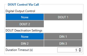
The scenario is activated and digital output is ON when a call is received from a number that is on the authorized numbers list.
