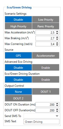
When vehicle parameters exceed the values of *Max Acceleration*, *Max Braking* or *Max Cornering* parameters, the scenario is activated: a record is generated, and the digital output status is changed to 1 when configured. You can configure all three parameters in m/s<sup>2</sup> units. The scenario is activated
