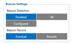
While selecting the **Beacons Detection** as **All**, the device will detect all beacons which are located around the device. Select **Beacons Detection** as the **Configured**, in this case, the beacons will only be detected and send if they were added to the Beacons List.
