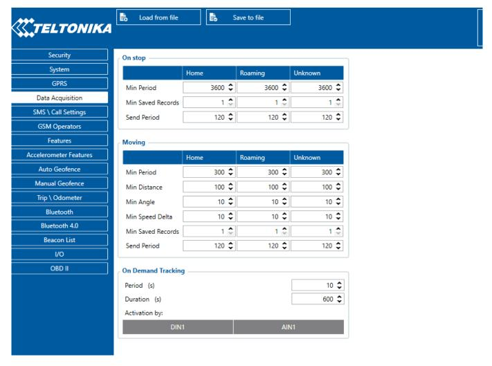
*Min Saved Records* defines minimum number of coordinates and I/O data that should be transferred within a single connection to the server. If FMM125 does not have enough coordinates to send to the server, it will check again after a time interval defined in *Send Period* field.
