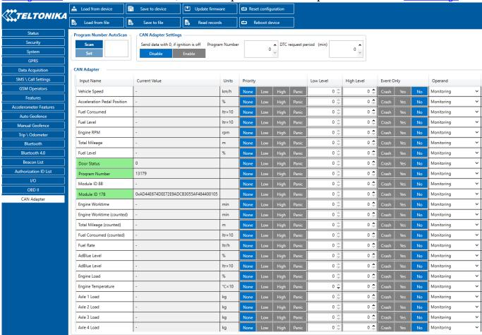
When using the offline configuration method user can select which CAN data (according to vehicle) will be sent directly to the server without connection to adapter.
