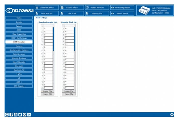
If roaming operator list is left empty, FMM130 will automatically detect home operator. If home operator is written to the roaming operator list, it will still be detected as home operator. Any operator not in the roaming operator list (except the home operator) will be recognized as unknown operator and FMM130 will work in Unknown mode (make sure it is configured to allow data sending – GPRS context is enabled).
