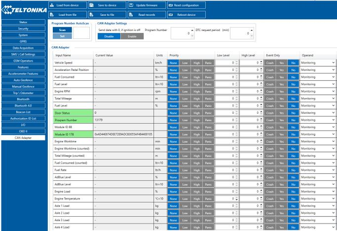
When using the offline configuration method user can select which CAN data (according to vehicle) will be sent directly to the server without connection to adapter.
