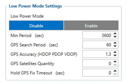
Low Power mode functionality was implemented to firmware from FMB.03.28.02.Rev.00. This functionality only works on devices that supports battery. It can only be active if device sleep mode is configured as Deep Sleep or Online Sleep. In other cases, low power mode is not allowed.
