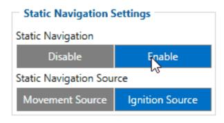
Static Navigation Mode is a filter, which filters out track jumps when the object is stationary.
