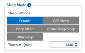
Backup Tracking both modes (Main and Backup) does not allow **Ultra Sleep** mode to be used so it has to be disabled in order for functionality to work effectively. Other sleep modes don't have an effect on the Bluetooth® functionality. If Ultra Sleep mode is selected - Backup Tracking options will be hidden and if Backup Tracking (Main or Backup modes) are selected then Ultra Sleep mode button will be hidden.
