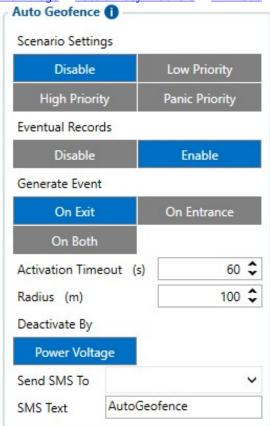
*AutoGeofence* is based on the last known position after the movement has stopped. You can be notified using this function if your car is taken away. The shape and size of Geofence zones are set by parameters. It is possible to state whether entering or leaving the geofence triggers an asynchronous message. AutoGeofencing options can be configured by following parameters as depicted in the right hand side figure:
