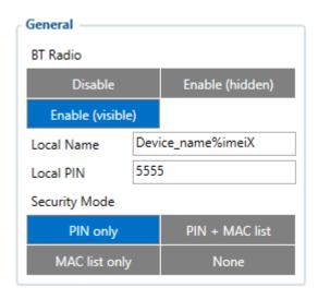
General functionality configures Bluetooth to work in slave mode. This mode allows any external device to connect to FMM800.
