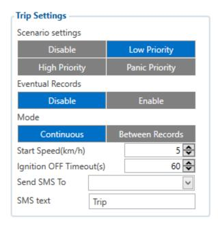
*Trip* section offers user to configure the *Trip* feature. *Trip* starts when Ignition according *Ignition* source is ON and Movement according *Movement source* is ON and also 'Start Speed' is exceeded. *Start Speed* defines the minimum GPS speed in order to detect *Trip* start.
