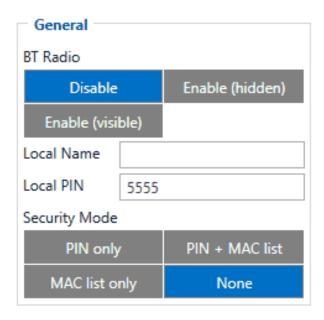
General functionality configures Bluetooth® to work in slave mode. This mode allows any external device to connect to FMM920.
