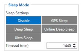
When in GPS sleep mode, FMM920 turns the GPS module off and continues making new periodic records. As a result power usage decreases, in turn saving vehicle battery.
