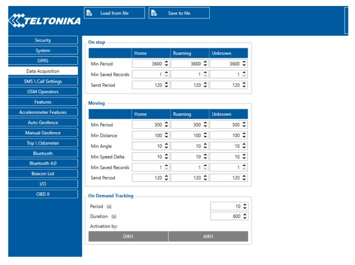
Min Saved Records defines minimum number of coordinates and I/O data that should be transferred within a single connection to the server. If FMU125 does not have enough coordinates to send to the server, it will check again after a time interval defined in Send Period field.
