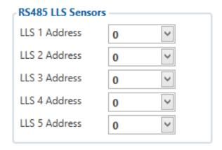
LLS addresses may be configured for 5 LLS sensors. If at least one LLS sensor is connected to FMU125 when configuring device using configurator, LLS sensor ID will be entered automatically.
