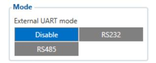
FMU-125 supports RS-232 and RS-485 serial standards and can be configured to work in different RS-232/RS-485 modes. More information about each mode is provided in RS-232 and RS-485. Only one mode may be selected at a time:
