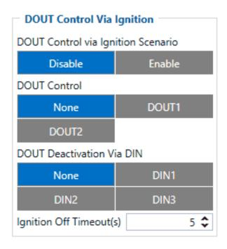
This feature allows direct control of DOUT by configured ignition source status. When enabled, the function will start to monitor ignition status, and once the ignition changes state from On to Off after configured Ignition Off a timeout, selected DOUT (Digital Output) will be turned On.
