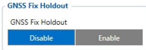
If this parameter is 'Enable', then for the first 30s of GNSS fix, coordinates are not considered valid. 'Disable' means that from the start of the fix coordinates are considered valid.
