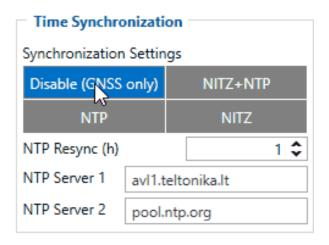
*Synchronization settings* is used for choosing the device's internal time synchronization source.
