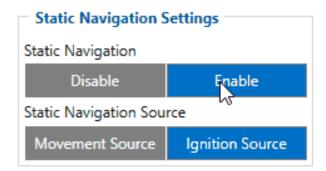
*Static Navigation Mode* is a filter, which filters out track jumps when the object is stationary.
