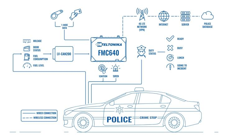
When installing FMC640 in a vehicle, follow the <u>mounting recommendations</u>. When connecting to the CAN bus, you must use the diagrams provided by our technical support engineers. The diagrams indicate in detail and clearly the connection points in the vehicle wiring and the required program number. FMC640 has the function of working with wireless BLE beacons and iButton reader via 1-wire.
