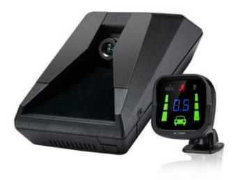
The collision warning system consists of the ADAS camera, which is mounted on the front window of the vehicle, and the Teltonika advanced GPS tracker FMC125, both connected via an RS-232 interface. ADAS camera detects alarming events in front and sends all the data to the dedicated server for further monitoring and analysis. Plus, it shows the Driver notification on events n front of the driver
