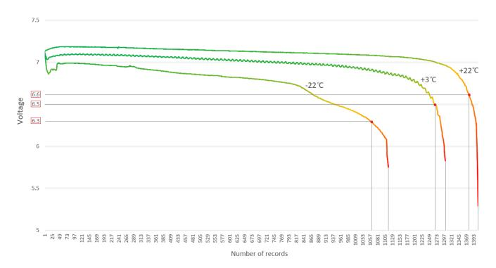
battery discharges more rapidly towards the end, but the device is capable of sending more records. The curve for lower temperatures maintains a more consistent decline before a sudden drop.
