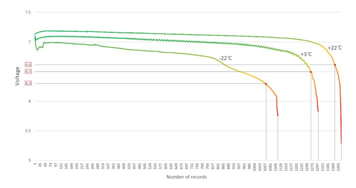
We advise against waiting until the device is fully depleted and suggest scheduling a battery replacement in advance. Based on the depicted curves, we recommend initiating device servicing when the following battery voltage values are received in your server:
