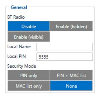
General functionality configures Bluetooth® to work in slave mode. This mode allows any external device to connect to TMT250.
