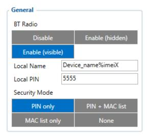
General functionality configures Bluetooth Bluetooth to work in slave mode. This mode allows any external device to connect to Bluetooth
