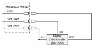
TTJ sensor pinout
