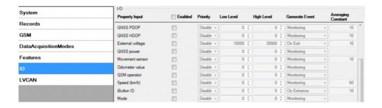
Enabled or disabled field – allows enabling I/O element so it is added to the data packet and is sent to the server. By default all I/O element are disabled and FM3612 records only GNSS coordinates.
