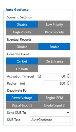
AutoGeofence is based on the last known position after the movement has stopped. You can be notified using this function if your car is taken away. The shape and size of Geofence zones are set by parameters. It is possible to state whether entering or leaving the geofence triggers an asynchronous message. AutoGeofencing options can be configured by following parameters as depicted in the right hand side figure:
