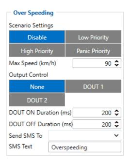
When vehicle speed exceeds configured maximum speed value the scenario is activated, an event record is generated and digital output status is changed to 1 when configured. Scenario is active until detected speed decreases below the set parameter value. info
