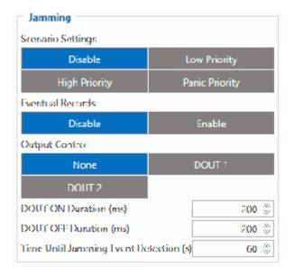
When GSM signal jamming is detected the scenario is activated, an event record is generated and digital output status is changed to 1 when configured once *Jamming* timeout runs out. If jamming ends during timeout countdown no event will be generated and output will not be controlled. *Eventual Records* parameter can be configured: when it is disabled scenario status value will appear in each AVL record, otherwise it will be appended only to eventual records. info
