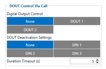
The scenario is activated and digital output is ON when a call is received from a number which is on the authorized numbers list.
