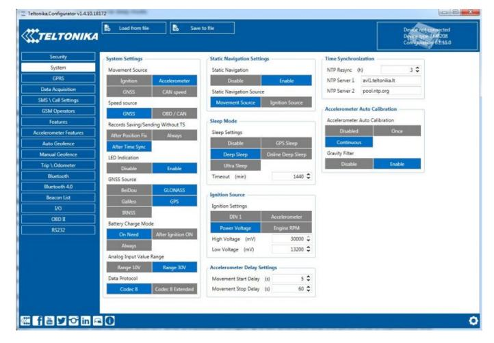
In GNSS Source settings user can configure which GNSS system(s) to use.
