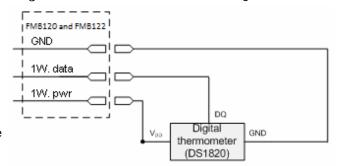
TTJ sensor pinout
