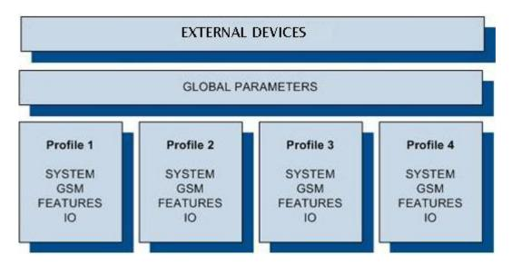
Switching between profiles (changing behaviour) can be performed by Profile switch depending on GSM operator code (mostly used for roaming applications), or by Profile switch depending on I/O event (on I/O value changing).
