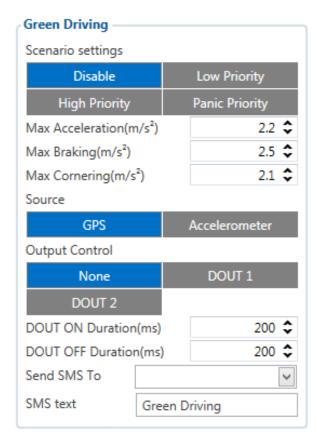
When vehicle parameters exceed the values of *Max Acceleration, Max Braking* or *Max Cornering* parameters, the scenario is activated: a record is generated and digital output status is changed to 1 when configured. You can configure all three parameters in m/s² units. Scenario is activated until current Acceleration, Braking or Cornering value decreases below the set parameter value. Parameters used with *Green Driving* functionality are given in a table below.
