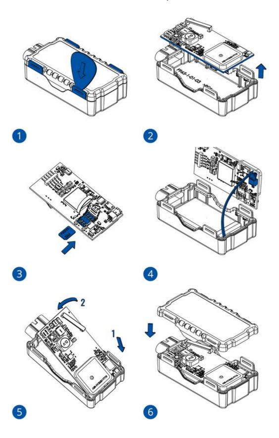
Nano-SIM card insertion/removal must be performed when device is powered off - external voltage and internal battery disconnected. Otherwise Nano-SIM card might be damaged or device will not detect it.
