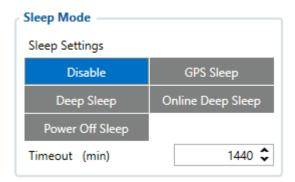
When in GPS sleep mode, FMM6YX turns the GPS module off and continues making new periodic records. As a result power usage decreases, in turn saving vehicle battery.
