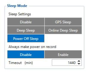
When the **Always make power on record** is enabled, the the device will make a record and send when waking up from external interrupt. Device goes into power off state where module is powered off to save maximum amount of power and can only wake if there is movement by accelerometer, external power is applied, ignition (DIN1) is detected, or it is time to make the next periodic record.
