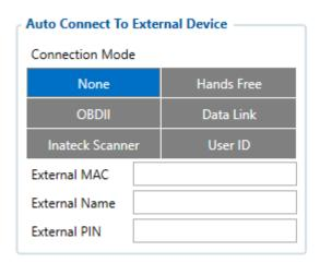
Auto connection functionality configures FMB1YX as master device, which allows connecting FMB1YX to an external device. FMB1YX currently supports these modes:
