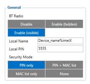
General functionality configures Bluetooth to work in slave mode. This mode allows any external device to connect to FMB1YX.
