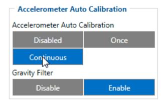
Users can disable or enable Accelerometer Auto Calibration and Gravity Filter features. This feature is available from firmware version 03.25.07.Rev.00. Under Accelerometer Auto Calibration settings, user can choose:
